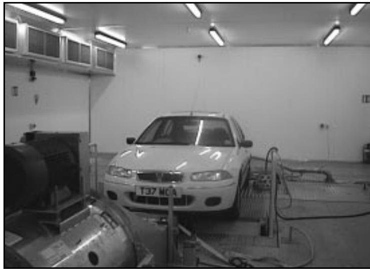
**Figure 3-1 The CVT Equipped Rover 216GSi on the Chassis Dynamometer**
